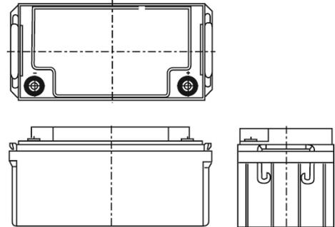
This battery type must never be installed suspended by their handles
